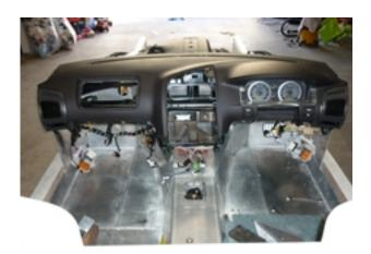
John has spent the last weekend working on getting the Falcon Dash into the Cobra shell. It will take some work to intergrate the Air Conditioning into the new dash area, but he's confident it will be completed in the next week.
